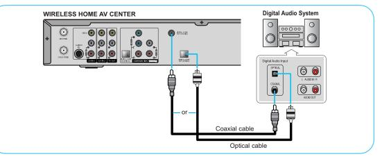
If your audio system has a coaxial digital audio input, connect to the "COAXIAL" output jack on the WIRELESS HOME AV CENTER.
